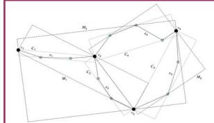
An example graph G with 4 edges  $e_1, ..., e_4$  and 4 vertices  $v_1, ..., v_4$ . The edges are represented as strip trees, with  $C_1, ..., C_4$ representing the root bounding boxes for each strip tree. The strip trees are merged bottom up in pairs to construct the GStree.
