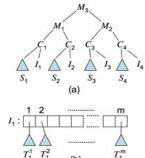
a)Each leaf C<sub>i</sub> points to the strip tree S<sub>i</sub> representing the graph edge e<sub>i</sub>, and to the corresponding moving object interval sets *l*<sub>i</sub>
