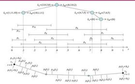
An example interval tree  $T_1^3$  for  $e_1$ . There are 11 intervals representing 11 moving objects during the time interval  $[t_2, t_3]$ . Moving objects  $p_1, ..., p_6$  are moving from vertex  $v_1$  to vertex  $v_2$ . Moving objects  $p_7, ..., p_{11}$  are moving in the opposite direction from  $v_2$  to  $v_1$ .
