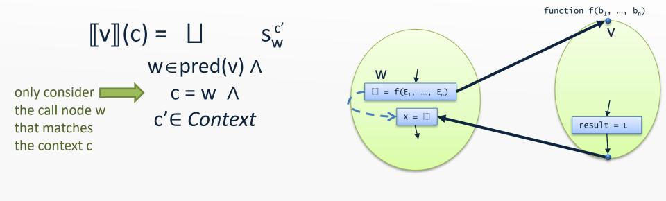
$s_{w}^{c'} = \begin{cases} \text{unreachable} & \text{if } \llbracket w \rrbracket(c') = \text{unreachable} \\ \bot [b_{1} \rightarrow eval(\llbracket w \rrbracket(c'), E_{1}^{w}), \dots, b_{n} \rightarrow eval(\llbracket w \rrbracket(c'), E_{n}^{w})] & \text{otherwise} \end{cases}$
